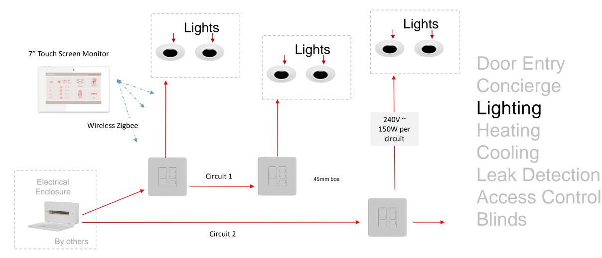
7" Touch Screen Monitor will control the lighting circuits through the gateway using Zigbee wireless technology. Note: the lights are 240V fed and power 240V LED lights up to 150W max per circuit
