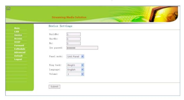
The settings of **building No** and **Unit No**. should be the same as that of corresponding outdoor panel No.
