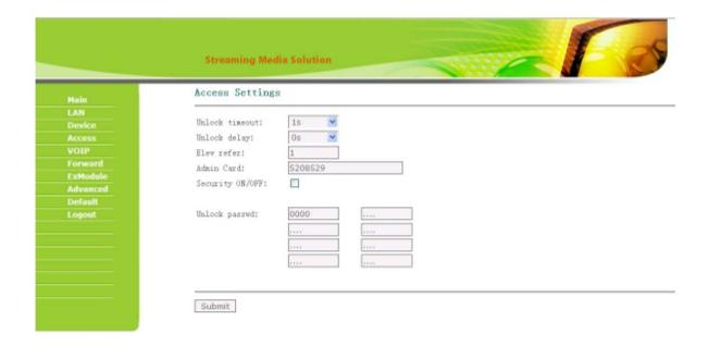
**Unlock timeout**: After 1-9 seconds, the door is closed.
