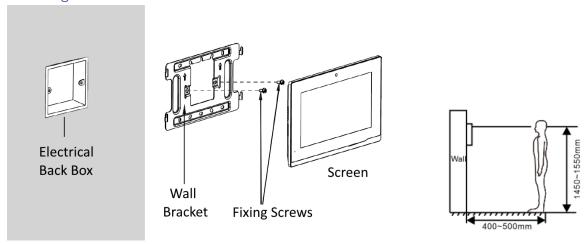
Best practice is to install the wall bracket onto an electrical Back Box.
