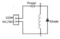
When connecting to an inductive load device such as a relay or electromagnetic lock, you are recommended to use a diode 1A/400V (included in the accessories) in anti-parallel with the load device to absorb inductive load voltage peaks. The intercom will be better protected in this way.
