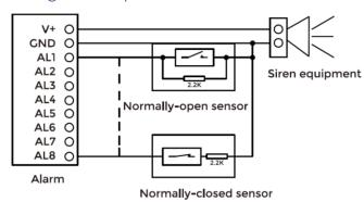
Using 2.2K resistors will instruct the Touch Screen Monitor to monitor the input connections.
