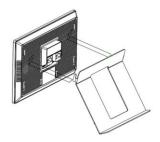
Insert the Metal base ORC-7T-E-DB into the top-hole inserts.
