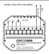
The room temperature is provided by the built-in sensor on the thermostat. An external 10k NTC sensor can be connected to the thermostat to provide additional temperature input. Externally sensed temperature is only readable on the Modbus.
