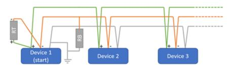
The "RB" going between "-" and "earth" is the "pull-down" resistor, the RT is required on larger installations.
