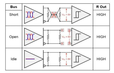
Modern transceivers have  $V_{IT+} \le 0V$  to ensure that the receiver outputs a failsafe HIGH during bus short, open, and idle events.
