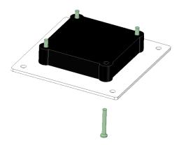
Line the reader holder up with the outer Studs and secure with washers and nuts.
