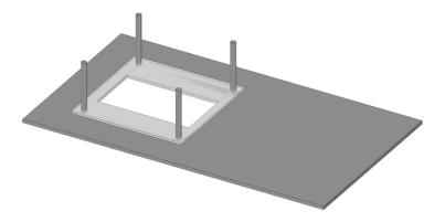
Pass cable through hole and mount bracket on rear of reader
