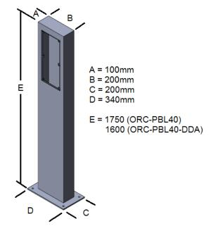
Typical installation - allow for floor to be above fixing bolts
