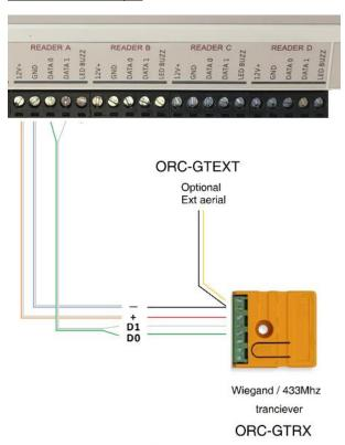
The ORC-GTRX is designed to allow Wireless RF gate Transmitters to pass through Wiegand to ORC-4DC Access Door Controller.
